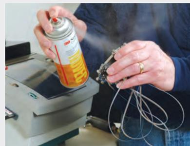
Applying contact cleaner to fixture with connectors.
