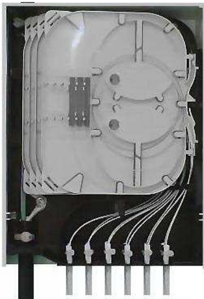
Internal view of PBPO 12 With 4 trays 1 slot, 6 Fibrlok 2540G mechanical splices. Out- let: 12 drops, 4 mm diameter 2 fibre cable
