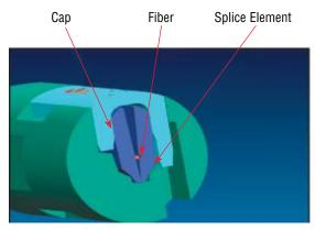
**Cross-sectional view of actuated splice**: After the fiber is inserted, the assembly tool depresses the cap to force clamping and locating surfaces against the fiber, locking and aligning the fiber in place.
