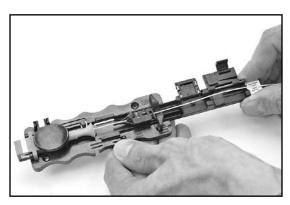
Optional: 3M<sup>™</sup> No Polish Connector can be tested in the tool using SC coupling.
