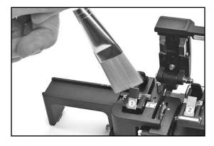
3.3 For 900  $\mu m$  buffer fiber, cut the buffer. If the 900  $\mu m$  slides easily from the fiber it is loose tube or semitight buffered fiber.
