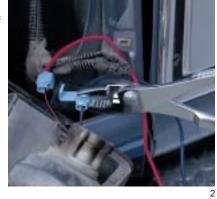
**Application:** Electrically connects two or three wire ends, insulates the connection, and provides a moisture resistant seal.
